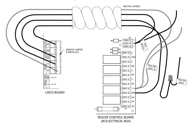
3. Connect the 39 inch black wire to the LWCO's terminal block at the **H** terminal. Run the wire through the conduit. In the electrical box, remove the wire from the circuit board's **R** connection in the small terminal block then twist that wire's end together with the black **H** wire from the LWCO and reinsert the twisted wire ends into the circuit board terminal block's **R** connection.
